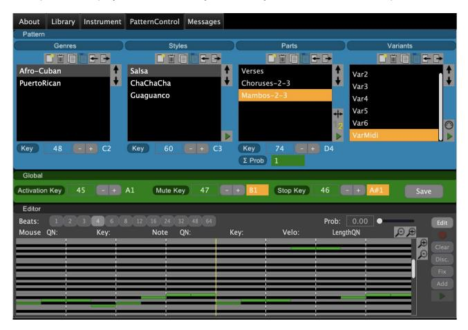
Find the actual pattern editor below the two test buttons. It can work in a (sort of) step sequencer mode or in a midi editor mode.
