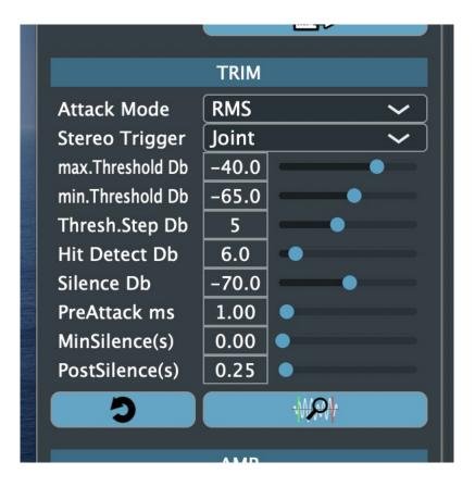
In this section you can set the parameters with which the attack / silence detection works. In most cases you should be able to detect suitable attack / silence positions with the default settings, adjusting only Max.Threshold dB and Silence dB.
